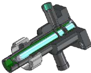
Unique Storage Chamber with Thorough Cleaning Technology, Wiper Ring with Backup seal for harsh media.
